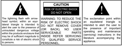
The Caution Marking may be located at the bottom enclosure of the apparatus.
